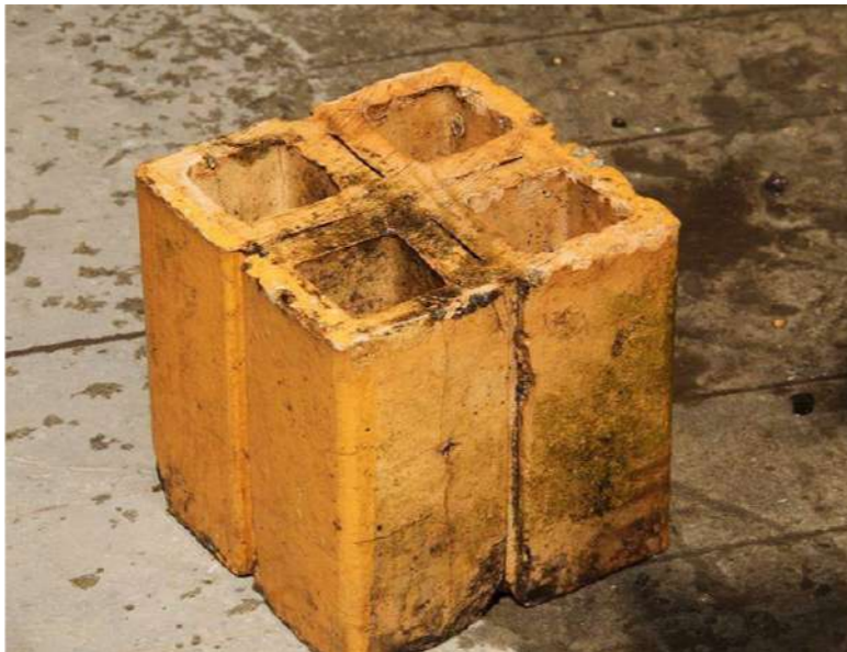
Typical masonry unit used to construct the walls to the laboratory and lecture buildings of Hlaing Campus
